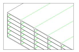
MARLON ST is the multiwall polycarbonate sheet manufactured by Brett Martin. The sheet is characterised high optical by clarity, light transmission, impact resistance and durability. It is available in a range of standard sizes, clear and tinted. MARLON ST Longlife has a coextruded UV protection layer on one side.
