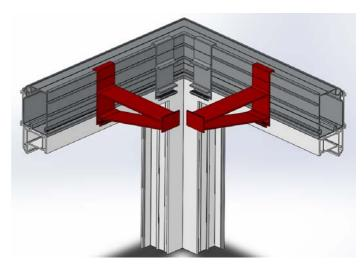
Once all brackets are in place screw them into position using 4.8 x 16(Min) self drilling screws.
