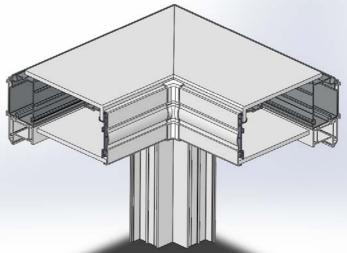
Clip into position the Faux Orangery Trim. The corners can be either mitred or square cut.
