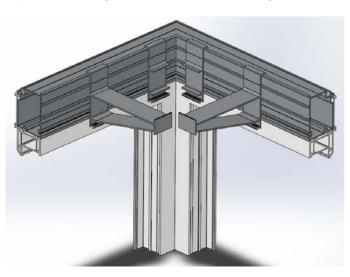
Locate the CB225 Capping board and screw into position.
